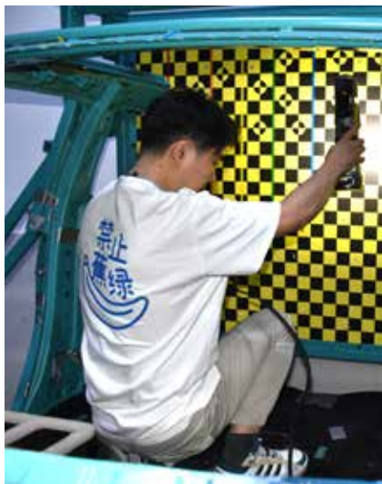
Tianlun Chen calibrates the volume in the passenger compartment ahead of a crash test.
